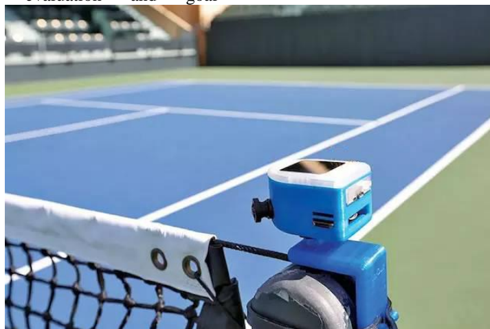
Figure 2 Intelligent acquisition equipment of tennis court.
